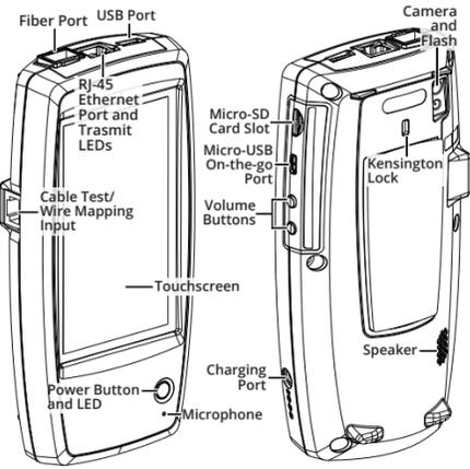
The LinkRunner G2 is an Android-based network testing and troubleshooting tool. It allows networking professionals to easily verify network availability and cable connectivity and to identify networks and ports. LinkRunner G2 can also act as a packet reflector for performance tests run by other NetAlly testers.
