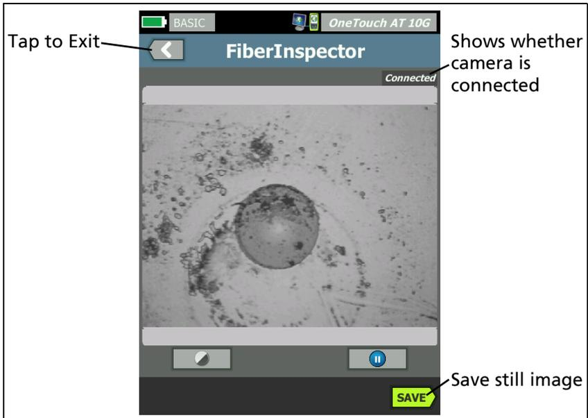
Figure 72. FiberInspector Image of an Endface
