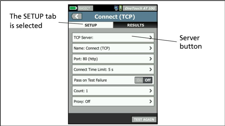
Figure 20. Connect (TCP) Test Setup Screen
