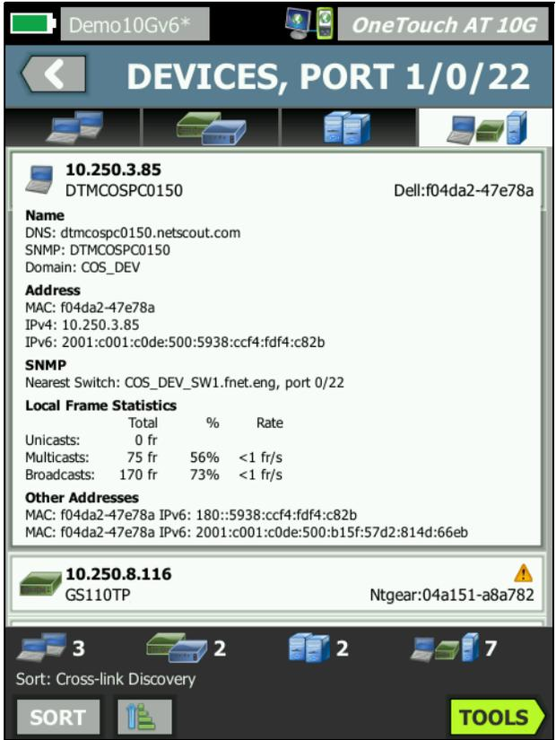
Figure 65. MultiPort - Device on Port Details Screen
