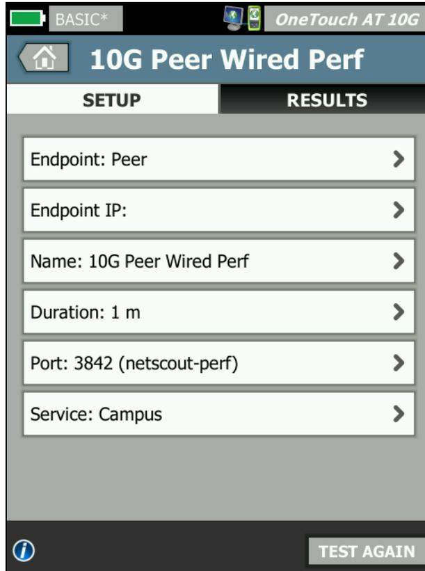
Figure 45. 10G Wired Performance Test Setup Tab Using Peer Endpoint
