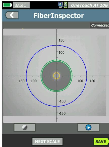
**Figure 73. FiberInspector Image with Measurement Scales**
