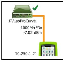
Figure 29. Fiber Cable Shown on HOME Screen
