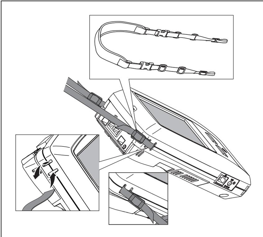
Figure 1. Install and Use the Hang Strap
