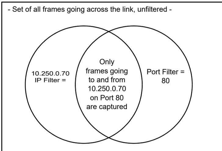
Figure 81. Capture Filters - Logical AND Operation
