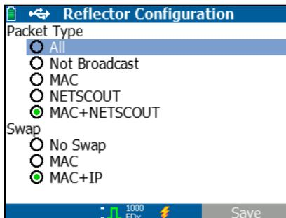
**MAC + NETSCOUT** - This filter setting allows the LinkRunner to only reflect frames when the destination MAC address field matches the LinkRunner's own MAC address and NETSCOUT payload.
