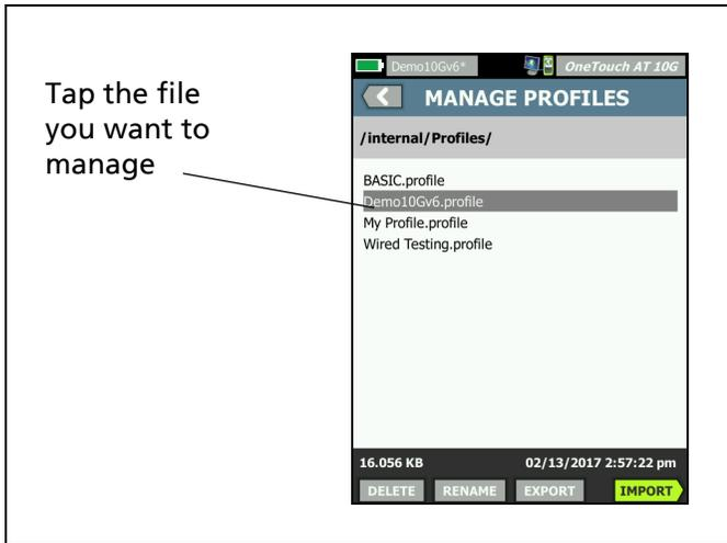
Figure 87. Manage Profiles Screen
