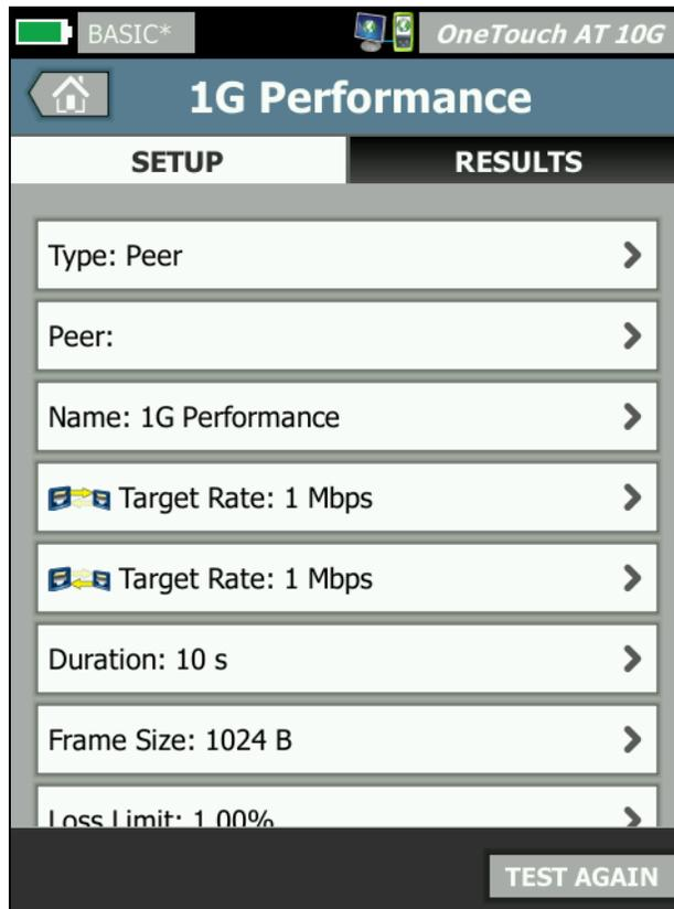
Figure 39. 1G Wired Performance Test Setup Tab
