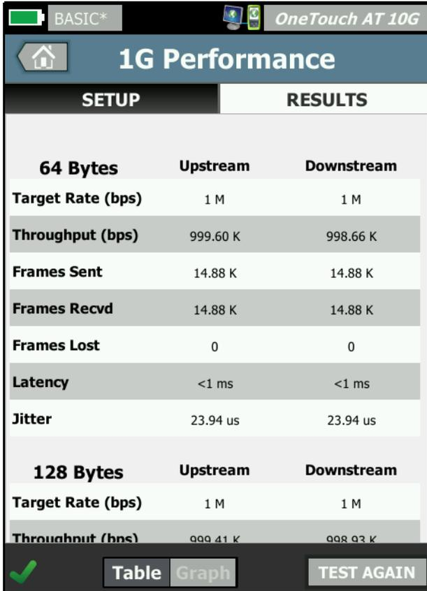
Figure 42. 1G Wired Performance Test (RFC 2544) Results
