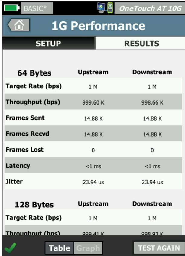
Figure 42. 1G Wired Performance Test (RFC 2544) Results
