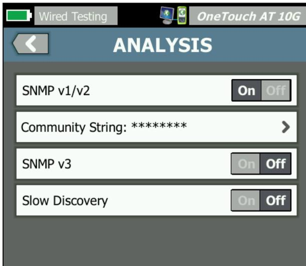
Figure 53. WIRED ANALYSIS Setup Screen
