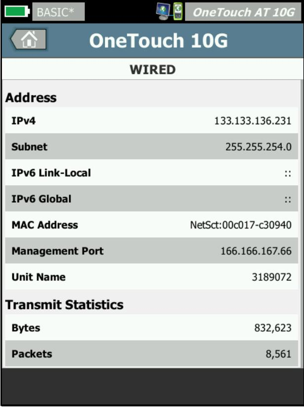
The screenshot shows the OneTouch AT 10G instrument interface. At the top, there is a status bar with a battery icon, the text 'BASIC\*', and icons for Bluetooth and Wi-Fi. Below this is a header with a home icon and the text 'OneTouch 10G'. The main content is titled 'WIRED' and is divided into two sections: 'Address' and 'Transmit Statistics'. The 'Address' section lists various network parameters, and the 'Transmit Statistics' section lists network performance metrics.
