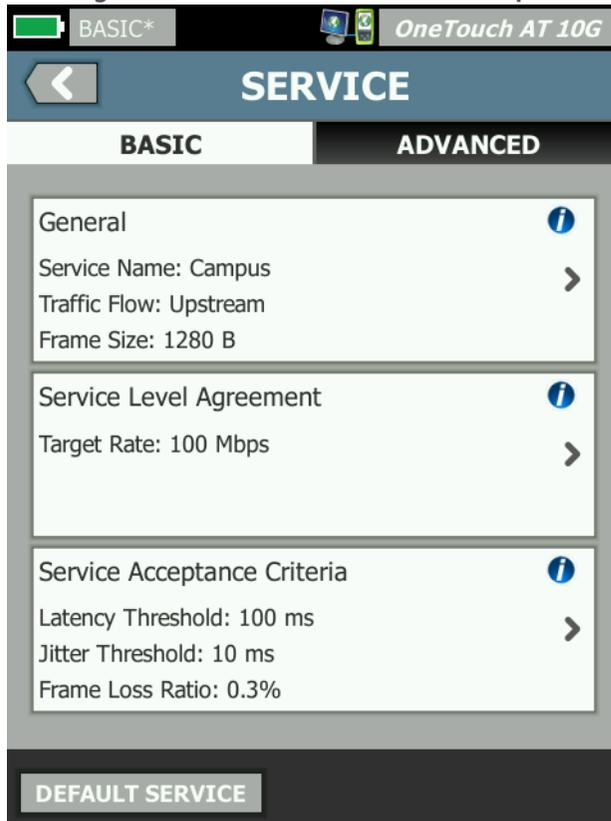
Figure 46. 10G Performance Peer/Reflector Service Configuration Screen
