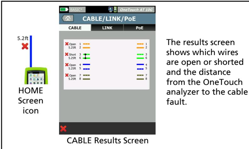
Figure 27. Underterminated Cable with Shorts and Opens
