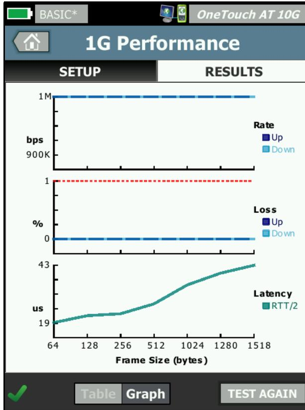
Figure 43. Wired Performance Test Results
