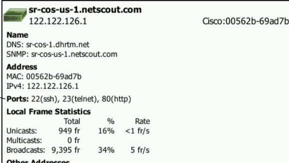
The screenshot shows the port scan results for the device 'sr-cos-us-1.netsecout.com' with IP address 122.122.126.1. The results include the device name, DNS, SNMP, MAC, IPv4, and open ports (22, 23, 80). It also displays local frame statistics for unicasts, multicasts, and broadcasts.
