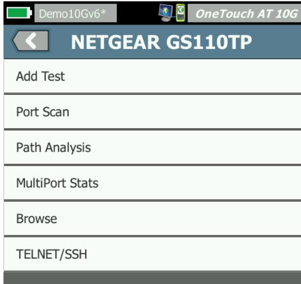
**Figure 61. MultiPort Statistics Button on Wired Analysis Tools Menu**
