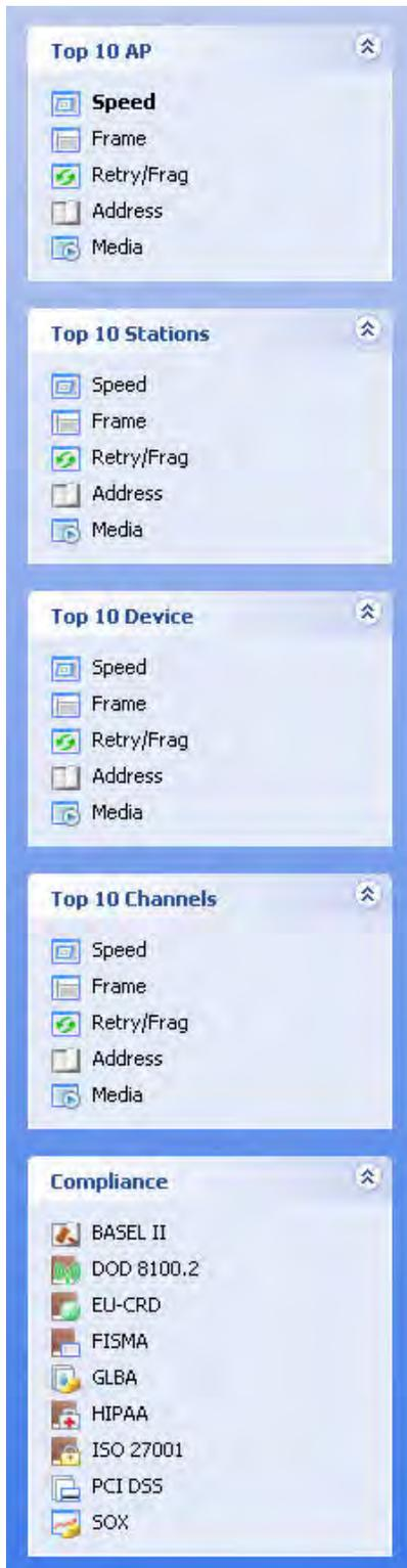
Each top 10 category can then be further divided by data type as shown in the Data Type drop-down list displayed under each section heading.
