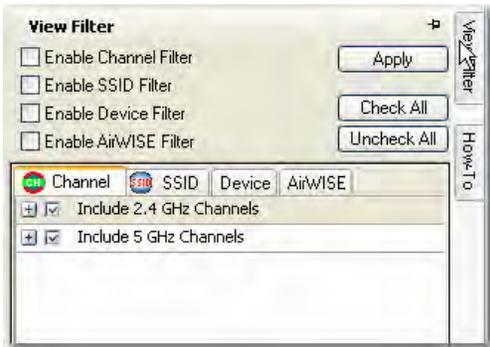
The View Filter pane automatically collapses when you click an area outside of it. You can anchor the pane to keep it visible by clicking the thumbtack icon in its upper-right corner.
