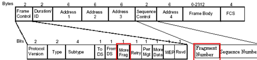
If the frames received are incomplete or invalid, the recipient device must transmit a retry frame so that the source device will re-send the data. While most wireless environments will experience a certain level of retry traffic, large quantities of retry frames can cause reduced throughput and may inhibit overall network performance.
