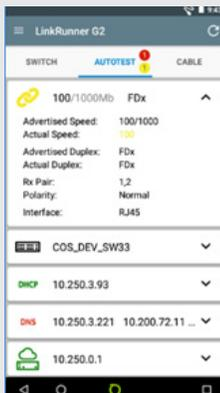
When connected to a switch at 10/100Mbps, the LinkRunner G2 can test for open on 4/5 or 7/8. A FAB (Floating Action Button) with an L will appear. Pressing the FAB will show the distance to the nearest open on the pair 4/5 or 7/8.
