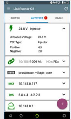
Verify voltage and the cable pairs used by a 24V PoE Injector.
