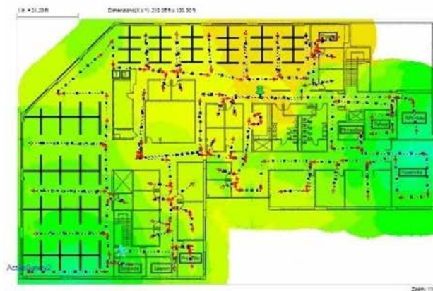
Signal strength heatmap generated with NetAlly's AirMagnet® Survey Pro
