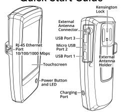
The AirCheck G2 is a comprehensive, handheld tool for network professionals to test and troubleshoot the latest wireless networks. The AirCheck G2 operates on 802.11b/g/n networks in the 2.4-GHz band and 802.11a/n/ac networks in the 5-GHz band. It offers the following test types:
