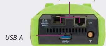
Main Ethernet Test Ports (RJ-45 & SFP)
