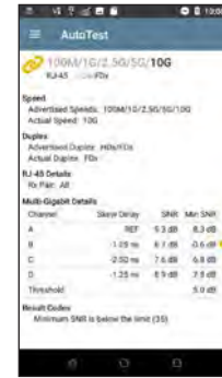
Cabling SNR measurement validates Multi-Gig links
