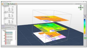
Automated WLAN Modeling using AirMagnet Planner
