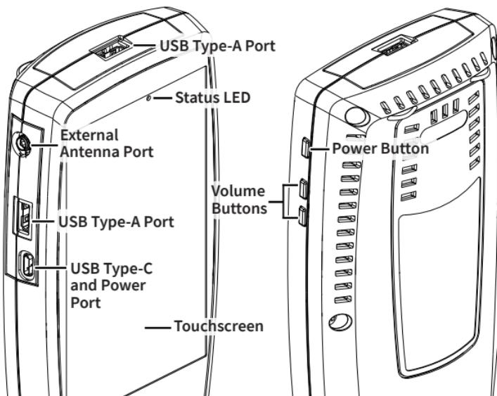
AirCheck G3 is a comprehensive, hand-held tool for testing and troubleshooting the latest wireless network technology. The AirCheck G3 operates on 802.11a/b/g/n/ac/ax networks in the 2.4 GHz, 5 GHz, and 6 GHz bands. It features applications from our AllyWare™ Common Technology platform for Wi-Fi device discovery and network analysis.
