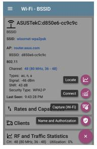
Tap Locate. This opens the Locate screen and causes your AirCheck G3 to "listen" for the BSSID or Client wireless devices you want to find using either the internal antennas or the optional external antenna (sold separately or in kits).
