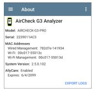
The About screen displays the model number, serial number, MAC addresses, software versions, SFP details, and current AllyCare contract status for your AirCheck G3.
