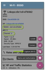
When the Capture app opens, filters are already set with the BSSID, Channel, and Channel Width from the Wi-Fi app.
