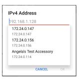
A drop-down list in the IPv4 Address dialog shows all the Test Accessories the AirCheck G3 has discovered through the discovery process, as well as any Test Accessories that are claimed to the same Link-Live organization as your AirCheck G3.
