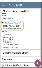
NOTE: If different Authorization statuses are assigned for different BSSIDs or MAC addresses on the same device, the Authorization of highest concern appears on the device's Details screens.
