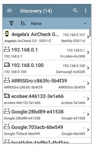
Like in AutoTest and other AirCheck G3 screens, the icons in Discovery change color to indicate a Warning or Failure condition. Discovery also displays device icons in Blue to indicate Problem-related information that does not constitute a warning or failure, and Green to indicate that a previous Problem has been resolved. (See the Problem Settings to adjust enabled Problems and thresholds.)
