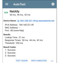
Device Name: DNS name of the device tested
