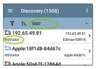
The selected Sort option displays in the Sort bar above the device list, and the sort characteristic for each device is shown under the device type icon. In the image above, all the devices associated with the "NSVisitor" SSID are sorted together. Individual devices on the same SSID are sorted numerically and alphabetically.
