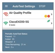
The Periodic AutoTest Status is summarized at the bottom of the AutoTest screens. Passes and failures are reported for each run of the entire Profile Group, rather than individual Profiles. Periodic AutoTests are skipped if the previous interval's test is still running when the next time interval occurs, such that the next run could not start.
