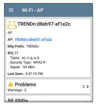
The Problems card shows the icon color of the highest severity problem, and the number of detected Warning, Failure, Information, and Resolved conditions for the device or network component.
