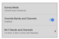
(Enabled for passive survey modes only.) Tap **Override Bands and Channels** to enable selection of different bands and channels than the values defined in **General Settings**. (These override settings are used only for AirMapper site surveys.) Enabling this setting displays the Wi-Fi Bands and Channels setting.
