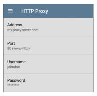
Tap each field to open a pop-up keyboard and enter the appropriate **Address** (you can enter a proxy name or an address), **Port** (set to match the proxy port), **Username**, and **Password**. Tap **OK** to save your entries.
