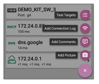
The Test Targets screen lists all of the defined and saved Test Targets. Checked boxes indicate the targets enabled in the current Profile. (Test Targets can be added to and used in any number of Wi-Fi Profiles.)
