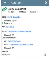
The Wi-Fi Link test screen shows these results:
