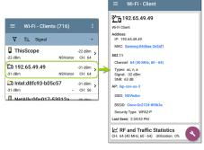
On the Wi-Fi Details screens, you can tap any blue linked name or address to open a Discovery or Wi-Fi app screen for the linked device
