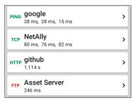
AutoTest Target tests are user-assignable endpoints to which AirCheck G3 attempts to connect each time the AutoTest profile runs. These tests ensure availability of internal or external websites, servers, and devices to users of your network.
