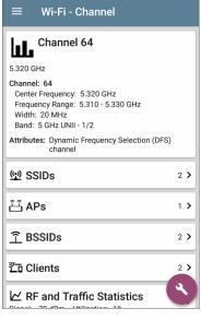
The Channel Details screen above shows how many SSIDs, APs, BSSIDs, and Clients are detected on Channel 64. Tap the lower cards in Wi-Fi Details to open a list screen that is filtered for the network component you are examining.
