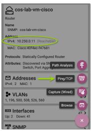
If you open the Ping/TCP app from this screen, the IPv4 address from the Discovery app is already configured as the Ping/TCP target.
