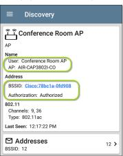
The user-assigned name for the AP and Authorization for the BSSID also appear on the Wi-Fi BSSID Details screen, as shown below.
