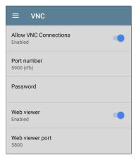
Allow VNC Connections: (Disabled by default.) Tap the toggle button to enable remote connections from VNC clients and display VNC options.
