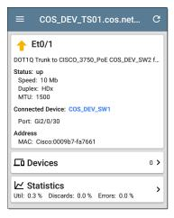
The Interface Details screen contains a description of the interface and information about its Status, Connected Device and Port, and Address
