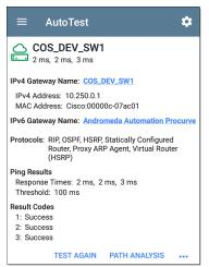
IPv4 Gateway Name: Resolved hostname of the Gateway or its IP address if no name could be discovered
