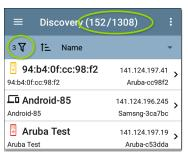
Back on the main Discovery screen, the screen title shows the number of filtered devices out of the total discovered devices (in the image above, 152 filtered devices out of 1308 total).
