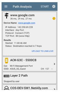
Like AutoTest, Path Analysis results are presented on cards. The top card shows the main test details, the second card shows information for the source device (your AirCheck
