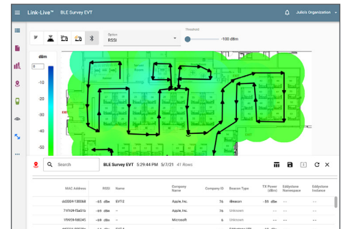
Bluetooth and BLE metrics that can be used to identify coverage and configuration problems.
