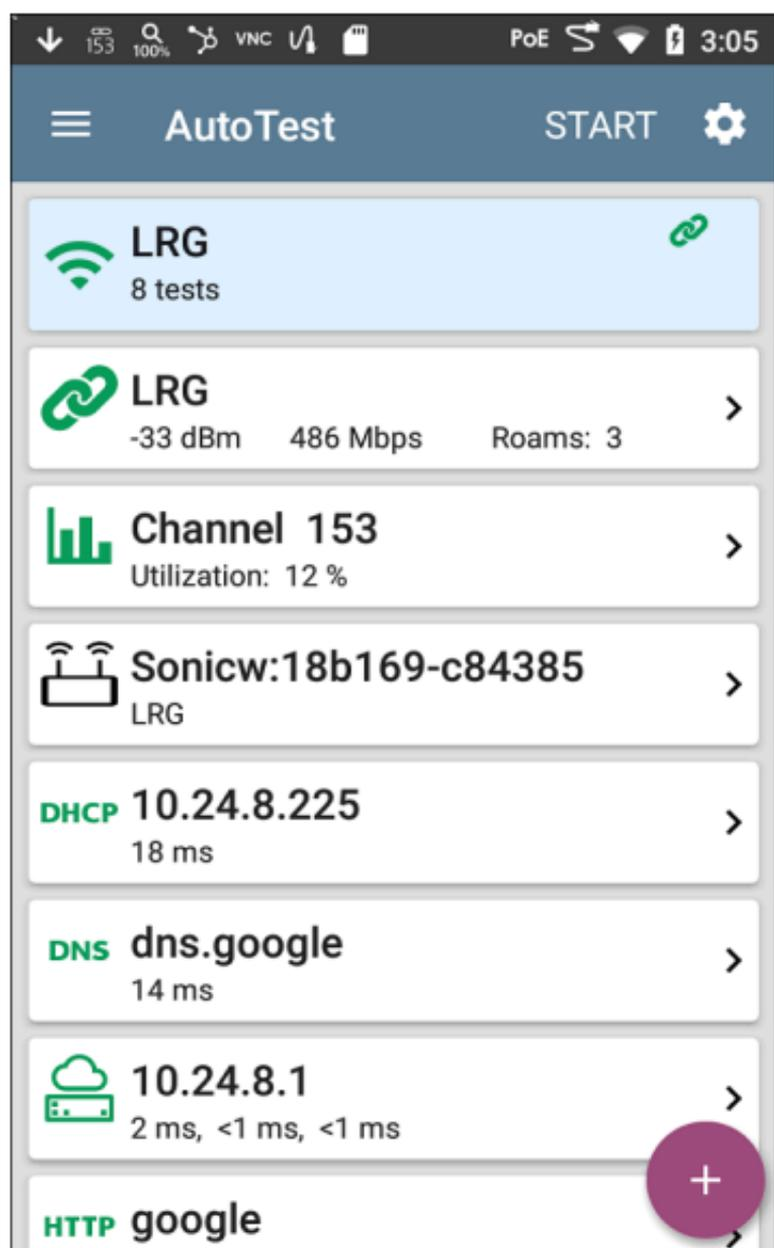
The screenshot displays the AutoTest application interface. At the top, there is a status bar with icons for signal strength, Wi-Fi, battery, and time (3:05). Below the status bar is a header with a menu icon, the text "AutoTest", a "START" button, and a settings gear icon. The main content area consists of several test result cards, each with a distinct icon and data:
