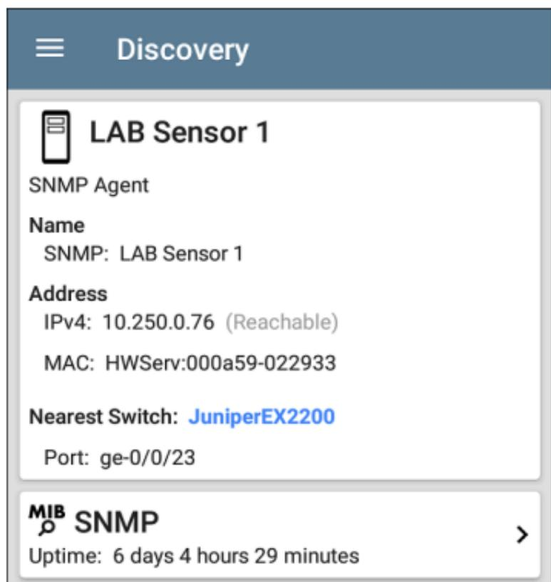
The screenshot shows a 'Discovery' interface with a menu icon on the left. The main content area displays details for 'LAB Sensor 1', which is identified as an 'SNMP Agent'. The details include the name 'SNMP: LAB Sensor 1', the address 'IPv4: 10.250.0.76 (Reachable)' and 'MAC: HWServ:000a59-022933', and the nearest switch 'JuniperEX2200' on port 'ge-0/0/23'. At the bottom, there is a section for 'MIB SNMP' with an uptime of '6 days 4 hours 29 minutes' and a right-pointing arrow.
