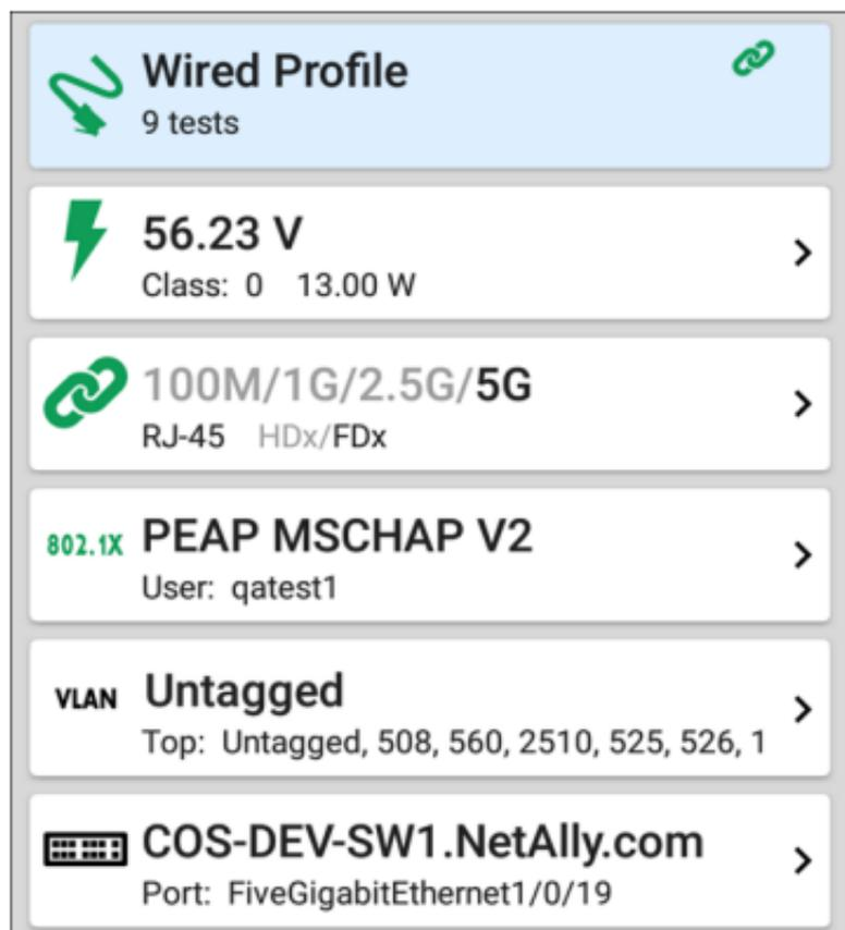
The screenshot displays a list of test cards for a 'Wired Profile' which contains 9 tests. The cards are as follows:
