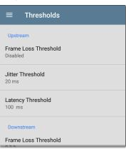
Tap each Threshold field to select or enter the maximum value allowed. If a measured value exceeds the threshold value, the test fails.
