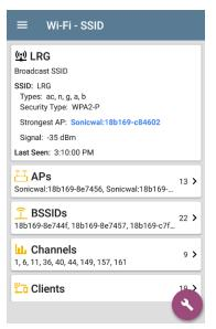
In addition to the Signal and Security Type, the SSID Details displays the AP on the network with the strongest signal, 802.11 Types that the APs in the network support, and the time the ESnXG CE last detected activity on the network (Last Seen).
