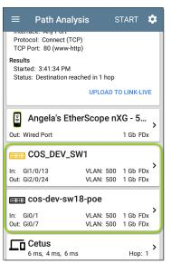
The ESnXG CE is able to identify these Layer 2 switches and their interfaces because it has configured SNMP access to the switches.
