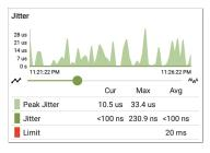
Jitter (Up/Down): Jitter is a measure of the variation in frame-to-frame latency in milliseconds
