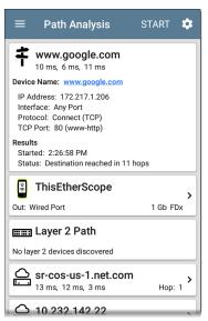
Like AutoTest, Path Analysis results are presented on cards. The top card shows the main test details, the second card shows information for the source device (your EtherScope nXG Controlled Edition), and the
