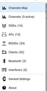
The Wi-Fi app's navigation drawer displays a real-time count (in parentheses) of each wireless component ESnXG CE has detected. Tap an option to open the corresponding screen.
