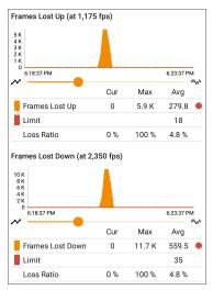
Frames Lost (Up/Down): Frame loss is quantified by the number of frames received subtracted from the number of frames sent.
