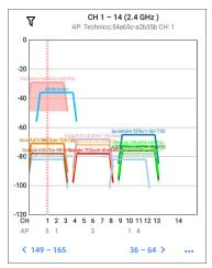
Double-tap the graph to zoom in or use "pinch" gestures with your thumb and forefinger. Tap the Restore icon is or reverse the pinch gesture to return to the full graph. The image below shows a zoomed-in view with the AP named "Technico:54a65ca2b35b" on channel 1 selected.
