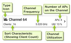
The lower left field displays the characteristic by which the list screen is currently sorted. In the image above, the Channels list is sorted by Client Count.
