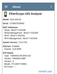
The About screen displays the model number, serial number, MAC addresses, software versions, SFP details, and current AllyCare contract status for your EtherScope nXG Controlled Edition.
