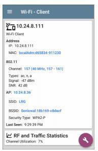
The top Client Details card for a connected Client displays the following information:
