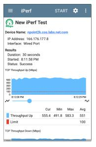
Test characteristics and status are displayed at the top of the iPerf results screen while the lower part of the screen displays a real-time graph of the TCP or UDP Upload and/or Download speeds. To pan and zoom on the graphs, you can swipe, double tap, and move the slider. See the Trending Graphs topic for an overview of the graph controls.
