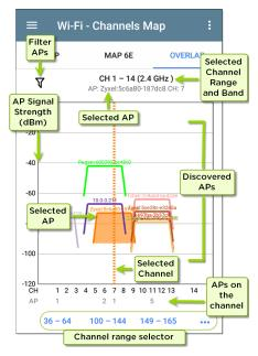
Tap the Filter icon near the top left to open the Overlap Filters screen to control what APs are displayed. You can select filters for channels, SSIDs, Signal, SNR, 802.11 type, or Security.
