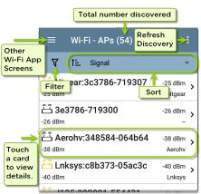
As with AutoTest and other ESnXG CE screens, the icons in Wi-Fi analysis change color to indicate a Warning or Failure condition. The app also displays icons in Blue to indicate Problem-related information that does not constitute a warning or failure, and Green to indicate that a previous Problem has been resolved.
