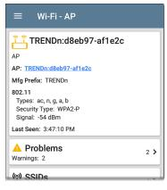
The Problems card shows the icon color of the highest severity problem, and the number of detected Warning, Failure, Information, and Resolved conditions for the device or network component.
