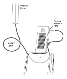
See the NXT-2000 Portable Spectrum Analyzer Instruction Sheet for more images and details of the External Antenna cable assembly.
