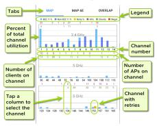
Blue vertical bars show the percentage of each channel's capacity used by 802.11 devices (light blue) and non-802.11 interference (dark blue). (EXG-200 only) If the Combine Utilization setting is enabled in General Settings, the graph shows only combined 802.11 and non-802.11 Utilization.
