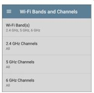
NOTE: Selecting a subset of channels and bands lets you exclude scans of unneeded channels from the survey. This improves survey performance and reduces the amount of data collected.
