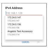
A drop-down list in the IPv4 Address dialog shows all the Test Accessories the ESnXG CE has discovered through the discovery process, as well as any Test Accessories that are claimed to the same Link-Live organization as your ESnXG CE.
