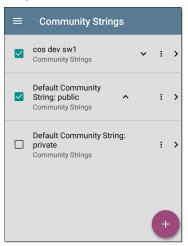
The ESnXG CE uses the checked strings in the order shown on this screen. If it does not receive a response from the queried device using one string, it sends the next string.
