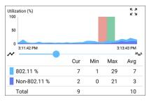
Retries (% of packets) graph: Plots percentage of transmitted packets that are retry packets
