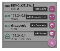
The Test Targets screen lists all of the defined and saved Test Targets. Checked boxes indicate the targets enabled in the current Profile. (Test Targets can be added to and used in any number of Wired or Wi-Fi Profiles.)
