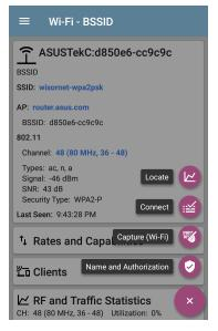
Tap Locate. This opens the Locate screen and causes your EtherScope to "listen" for the BSSID or Client wireless devices you want to find using either the internal antennas or the optional external antenna (sold separately or in kits).
