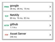
AutoTest Target tests are user-assignable endpoints to which EtherScope nXG attempts to connect each time the AutoTest profile runs. These tests ensure availability of internal or external websites, servers, and devices to users of your network.
