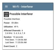
**Power**: The most recently observed power output from the device
