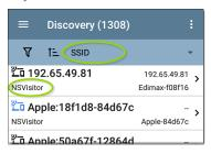
The selected Sort option displays in the Sort bar above the device list, and the sort characteristic for each device is shown under the device type icon. In the image above, all the devices associated with the "NSVisitor" SSID are sorted together. Individual devices on the same SSID are sorted numerically and alphabetically.
