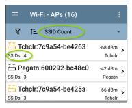
The selected Sort option displays in the Sort bar above the list, and the sort characteristic for each item is shown under the type icon and name. In the image above, the discovered APs are sorted by SSID Count, which is shown below each AP iron
