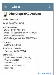
The About screen displays the model number, serial number, MAC addresses, software versions, SFP details, and current AllyCare contract status for your EtherScope nXG.
