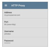
Tap each field to open a pop-up keyboard and enter the appropriate **Address** (you can enter a proxy name or an address), **Port** (set to match the proxy port), **Username**, and **Password**. Tap **OK** to save your entries.
