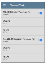
(EXG-200 only) If the **Combine Utilization** setting is enabled in **General Settings**, only a single, combined **Utilization Threshold** setting appears.
