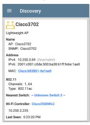
The linked and underlined Cisco MAC address in the screen image above opens the Wi-Fi app's AP Details screen, where you can view the other wireless attributes associated with the Lightweight AP. The Nearest Switch and Wi-Fi Controller links open a Discovery app Details screen for those devices.
