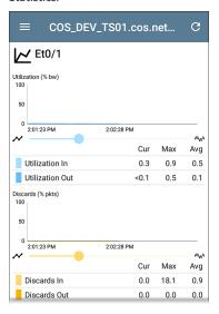
The Statistics screen displays real-time trending graphs of Utilization, Packet Discards, Packet Errors. See the Trending Graphs topic for an overview of the graphs' pan and zoom controls.
