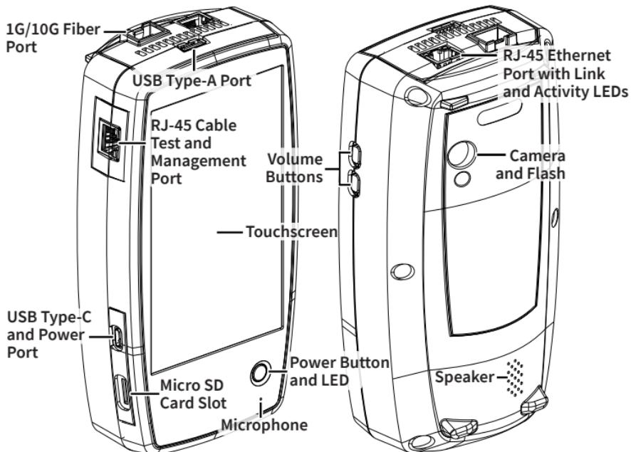
LinkRunner® 10G is a rugged hand-held tool for testing and analyzing wired copper and fiber Ethernet networks. This Multi-Gig Network Tester features applications from our AllyWare™ Common Technology platform for wired network measurement and validation.
