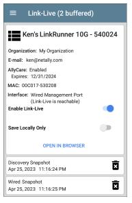
The buffered files displayed automatically upload to Link-Live.com once your LR 10G connects to an active network.
