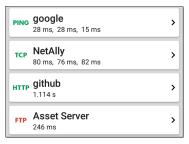
AutoTest Target tests are user-assignable endpoints to which LinkRunner 10G attempts to connect each time the AutoTest profile runs. These tests ensure availability of internal or external websites, servers, and devices to users of your network.
