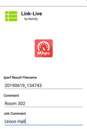
The Link-Live sharing screen opens and allows you to revise the auto-generated file name and attach comments to the iPerf result, which is displayed on the Results page on Link-Live com.
