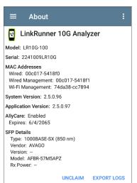
The About screen displays the model number, serial number, MAC addresses, software versions, SFP details, and current AllyCare contract status for your LinkRunner 10G.
