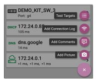
The Test Targets screen lists all of the defined and saved Test Targets. Checked boxes indicate the targets enabled in the current Profile. (Test Targets can be added to and used in any number of Wired Profiles.)
