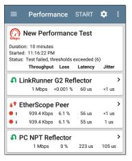
Performance results update every five seconds if you are using only Reflector endpoints, and/or a Netally tester Peer running v1.2 or newer software, with a test Duration of 4 hours or less. If you are running a 10 second test, all results display after 10 seconds. Otherwise, results update every 30 seconds.
