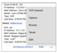
Tap TCP Connect to open the corresponding NetAlly apps, populated with the switch's address.
