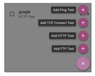
Tap any target test name to open that test's settings. You can then enter a custom test name, target address, or thresholds. For more information on settings, see:
