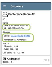
NOTE: If different Authorization statuses are assigned for different MAC addresses on the same device, the Authorization of highest concern appears on the device's Details screens.
