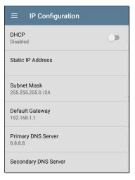
The Static IP address fields for **Subnet Mask**, **Default Gateway**, and **Primary** and **Secondary DNS Servers** only appear if DHCP is disabled. Tap each field to open a pop-up number pad and enter the static addresses as needed. Tap **OK** to save your entries.
