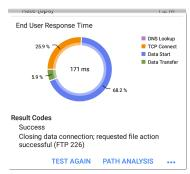
**End User Response Time**: Pie chart of the times for each phase of the test (DNS Lookup, TCP Connect, Data Start, and Data Transfer).
