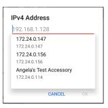
A drop-down list in the IPv4 Address dialog shows all the Test Accessories the LR 10G has discovered through the discovery process, as well as any Test Accessories that are claimed to the same Link-Live organization as your LR 10G.
