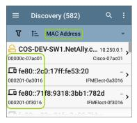
The selected Sort option displays in the Sort bar above the device list, and the sort characteristic for each device is shown under the device type icon. In the image above, all devices are sorted in order of the MAC Address.
