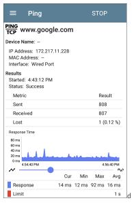
The graphs update in real time and then save and display data for up to 24 hours (depending on test type and/or link status).
