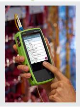
The EtherScope nXG is a portable network expert, easy to use for network technicians, but powerful enough for network engineers. As a multi-technology, all-in-one handheld network analyzer, it enables engineers and technicians to get more done faster, from deployment to maintenance, troubleshooting, and documentation of their ever-changing Wi-Fi and Ethernet access networks.
